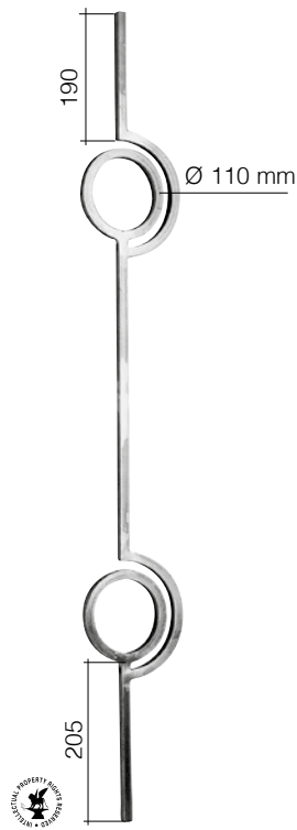
Art. 1091/2 \varnothing 12 mm L 135 mm H 1000 mm
